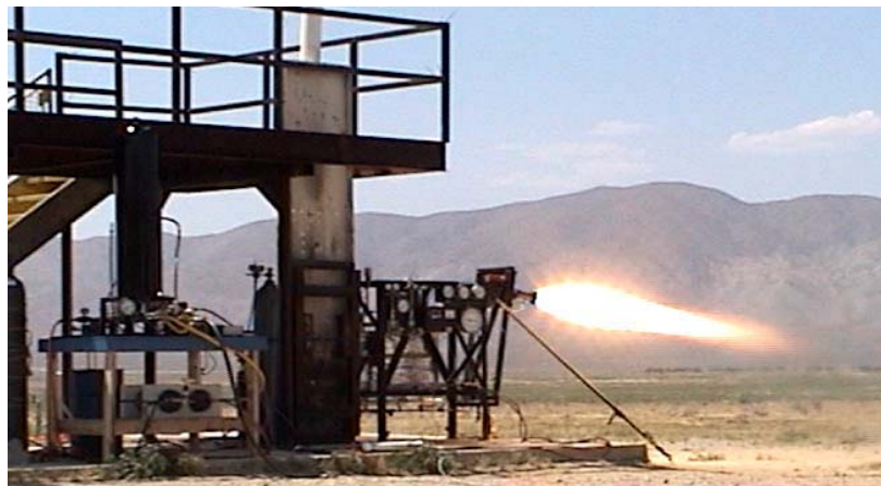
Figure 2 Atlas Vernier Engine Running with Fuel Pumped and LOX Pressure-fed. (Test facility courtesy Reaction Research Society)
