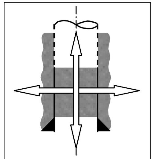
Steel tubular is not an acceptable permanent WBE unless it is supported by cement, or a plugging material with similar functional properties as listed above, (inside and outside).
