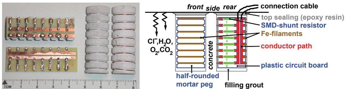
**Figure 1.** Front and reverse side of prototypes of 8-wire filament-sensor with prefabricated mortar pieces; two semicircular sensors can be installed together in one drillhole
