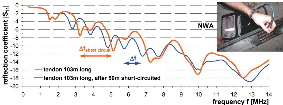
Figure 4. In-situ-ERM-measurement at a 103m long external bridge tendon: measured reflection coefficient  $|S_{11}|$  of an unbroken strand with and without electric short circuit after 50m simulating a local fracture; the photo shows the measurement configuration
