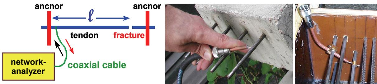
Figure 3. ERM: Measurement principle and external resp. internal coupling adapters
