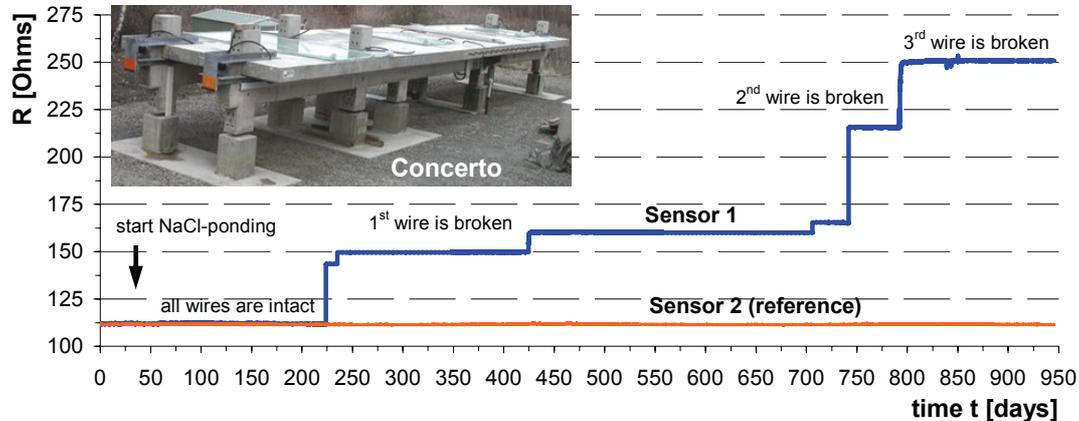
**Figure 2.** Measured sensor resistance  $R$  of two subsequent installed 8-wire filament sensors with 0.065mm thin iron wires installed in the slab of the 18.5m long trial bridge “Concerto” (see photo), only sensor 1 has been exposed to 0.5mol NaCl-solution
