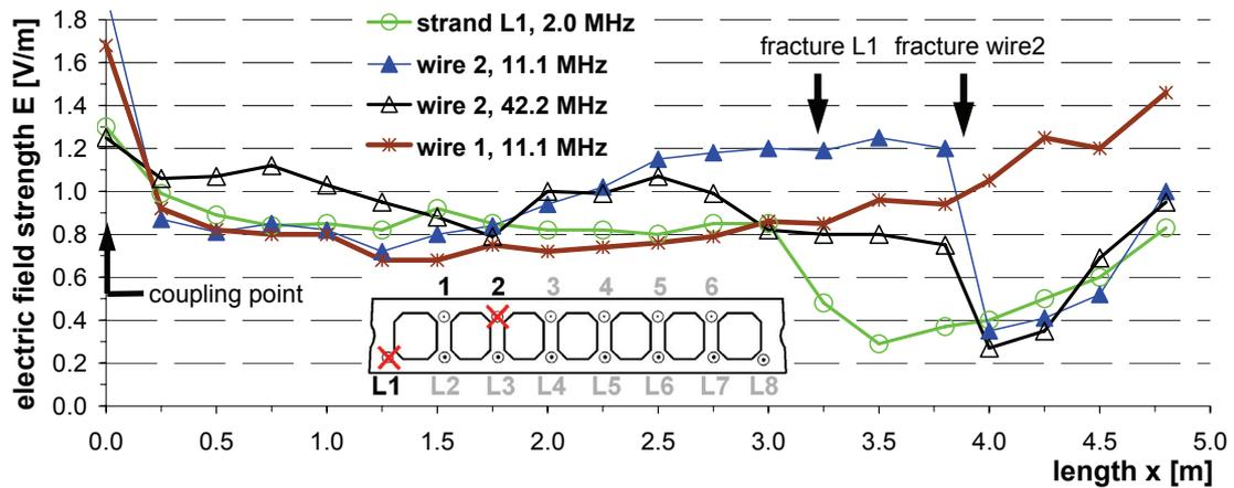
**Figure 5.** Electric field strength data from the upper surface of a 4.8m long prestressed hollow slab with cross section of the member, only wire 1 is unbroken; the static field strength  $E_0$  was determined to 0.05-0.10 V/m
