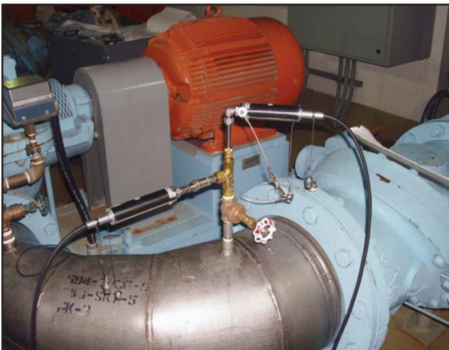
Figure 1: PUMP TESTING EQUIPMENT USING THERMODYNAMIC METHOD
